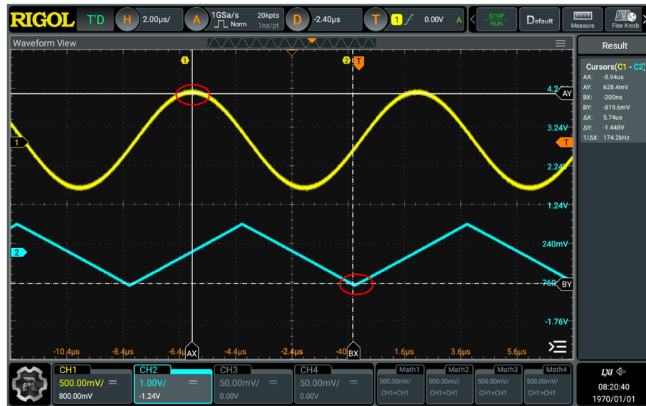
Figure 10.13 Track Measurement (after Horizontal Expansion)
